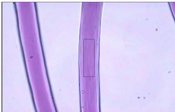
Camera picture of fibre, the frame marks the actual size of the analysed area.
