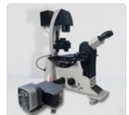
DSD Uni with Leica DMI6000
