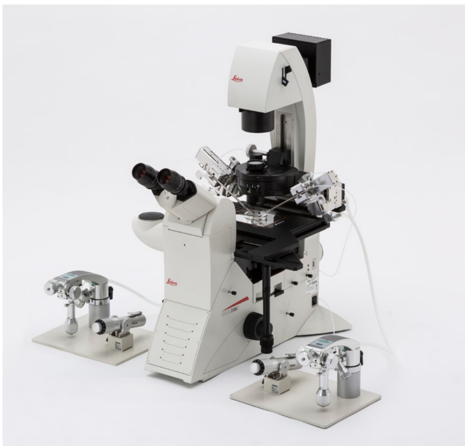
A perfect ICSI workstation: Leica DMi8, 3-plate stage, condenser S40 for modulation contrast for objectives 5x to 63x, Narishige Takanome® micromanipulator with injection units, heating stage 37°C.
