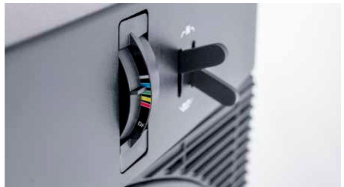
The aperture diaphragm's scale on the incident-light axis has color markings matching the objective color codes.
